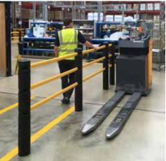
Conforms to OSHA Standard 1910.23 for guarding floor and wall openings with railing and to IBC Standard 1012 regarding handrails, including section 1012.3 concerning the ability to grasp handrails.
